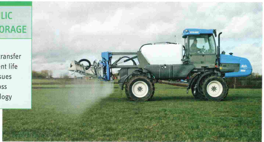
As illustrated in the 'Hydraulic Hybrid Drive' diagram, hydrostatically driven sprayers are particularly suited to utilising hydraulic energy storage technology. On acceleration, pressurised oil helps to drive the wheel motors.
