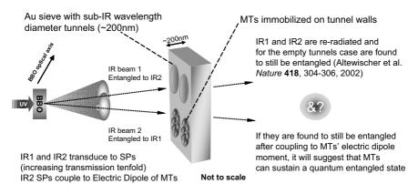
Fig. 7.2. For certain orientations, a UV photon is absorbed by the BBO crystal and reemitted as two entangled IR photons (IR1, IR2). One of the EPR-paired beams can be allowed to undergo the quadruple transduction of photon  $\rightarrow$  surface plasmon  $\rightarrow$  electric dipole moment  $\rightarrow$  surface plasmon  $\rightarrow$  photon while the other beam can either be left undisturbed or undergo any subset of transductions determining whether proteins can sustain entanglement.
