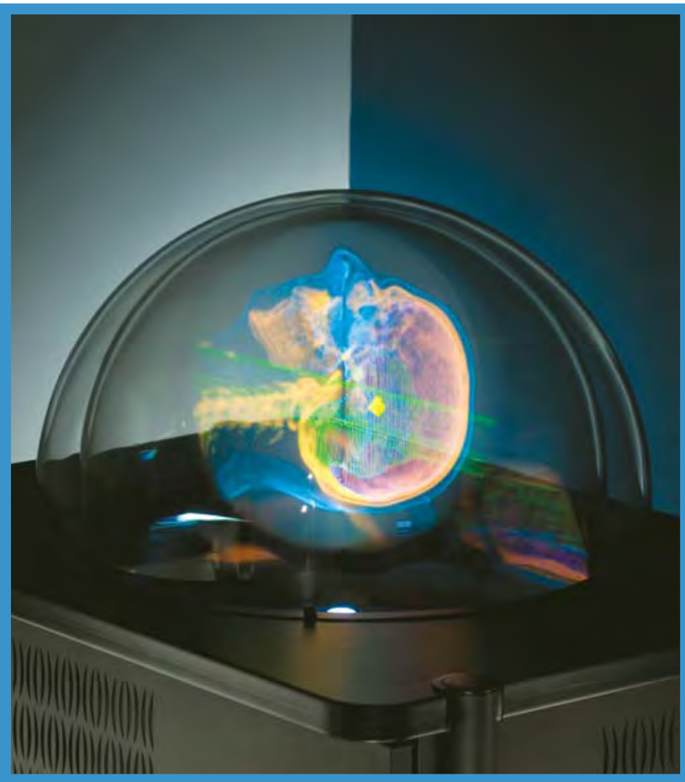
ANGLE OF ATTACK: Data from a CT scan is projected in 3-D in PerspectaRad, revealing a brain tumor core (yellow diamond, center) and possible paths for radiation treatment (green rays).
