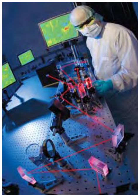
SOLID-STATE LASER is tested at Northrop Grumman Space Technology. A high-power version of such a device—capable of generating 100 kilowatts or more—could enable ground troops to destroy incoming mortars or rockets.
