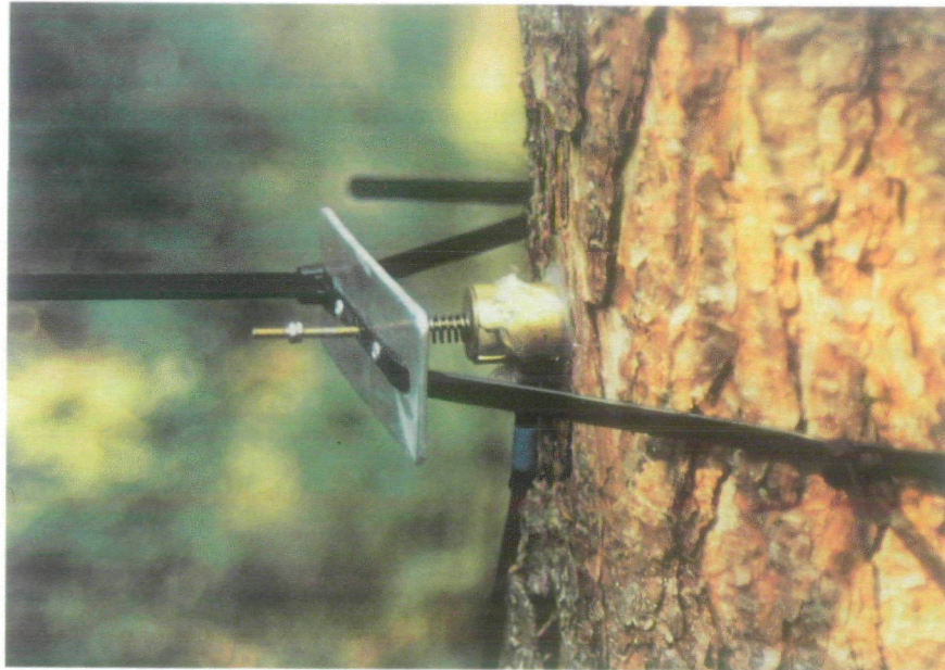
Fig. 3. Ultrasound acoustic emission sensor (I151) operating on a mature Scots pine tree. A hole is made in the bark, and the phloem and cambium layers beneath are removed so that the sensor is attached directly to the xylem (wood) beneath.
