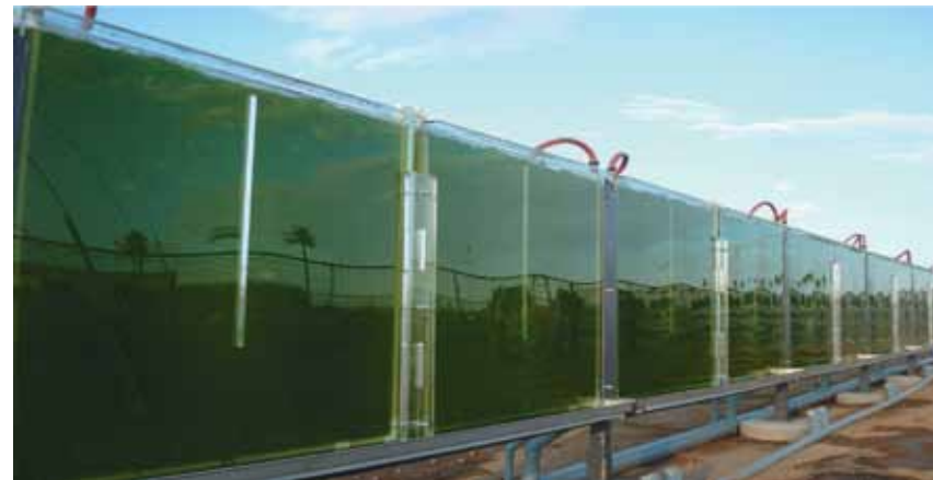
▲ Figure 10.3 Alternative fuels from algae. The power of sunlight can be tapped to generate a sustainable alternative to fossil fuels. Species of unicellular algae that are prolific producers of plant oils can be cultured in long, transparent tanks called photobioreactors, such as the one shown here at Arizona State University. A simple chemical process can yield “biodiesel,” which can be mixed with gasoline or used alone to power vehicles.
