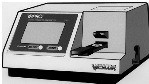
FIG. 18.14 The vapor pressure osmometer made by Wescor, Inc., Logan, Utah. (From a Wescor, Inc., Logan, Utah, brochure. Reprinted by permission of Wescor, Inc., Logan, Utah.)
