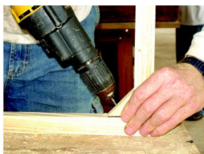
Figura 28 - Parafusando as bandejas
