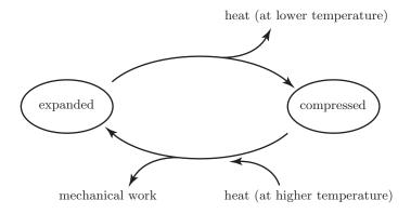
Figure 6.6: (Diagram.) Operating cycle of a heat engine.
