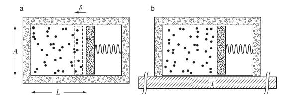
Figure 6.4: (Schematics.) Compression of gas by a spring. The direction of increasing  $\delta$  is to the left. (a) Thermally isolated system. (b) Subsystem in contact with a heat reservoir, at temperature T. The slab on the bottom of (b) conducts heat, whereas the walls around the box in both panels (hatched) are thermally insulating. In each case the chamber on the right (with the spring) contains no gas; only the spring opposes gas pressure from the left side.
