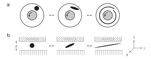
Figure 5.2: (Schematics.) Shearing motion of a fluid in laminar flow, in two geometries. (a) Cylindrical (ice-cream maker) geometry, viewed from above. The central cylinder rotates while the outer one is held fixed. (b) Planar (sliding plates) geometry. The top plate is pushed to the right while the bottom one is held fixed.
