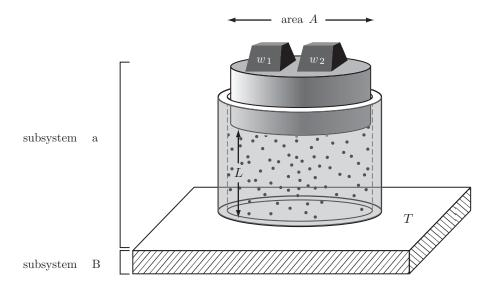
Figure 6.5: (Schematic.) Extracting mechanical work by lifting a weight. After we remove weight  $w_2$ , the cylinder rises, lifting weight  $w_1$ . A large thermal reservoir (subsystem B) maintains the cylinder at a fixed temperature T.
