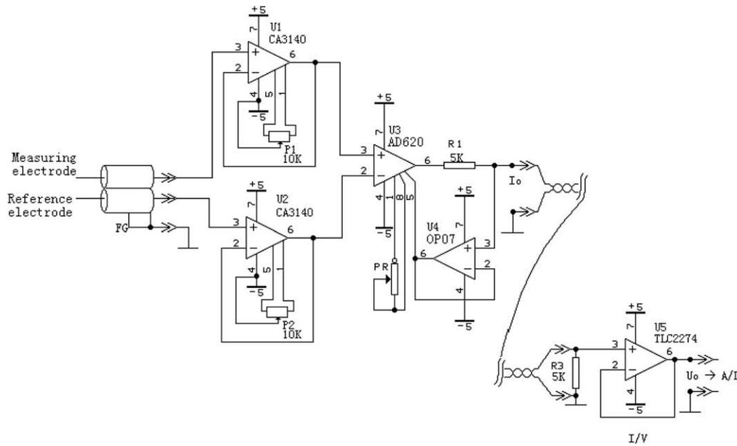
Fig. 2 – Preamplifier and voltage/current converter circuit for electrical signals in plants.
