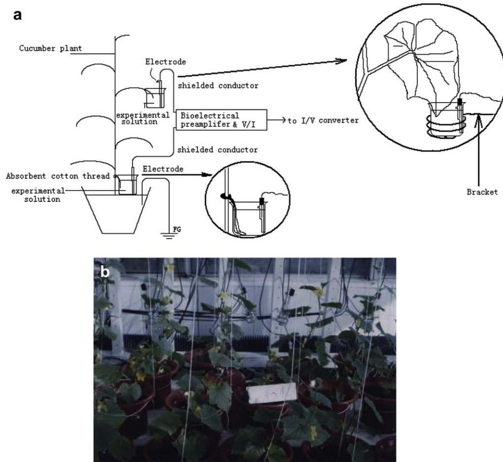
**Fig. 1 – (a) Experimental setup for detecting electrical signals in plants. FG (frame ground, i.e. the earth). (b) Measuring the electrical signals in plants in the greenhouse.**
