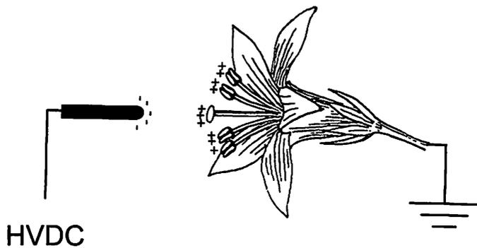
**Fig. 4. The system used for determining the detaching force imposed by a pin electrode hooked to various potentials. The scheme illustrates the mechanism of inducing charge and exerting force on a grounded object.**
