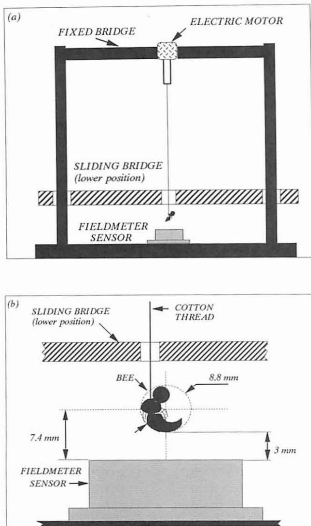
Fig. 2. Experimental setup for measuring the charge on a bee; the bridge is lowered to retain the bee above the field meter during the measurement. (a) General view and (b) the geometrical arrangement of the bee and the field meter.
